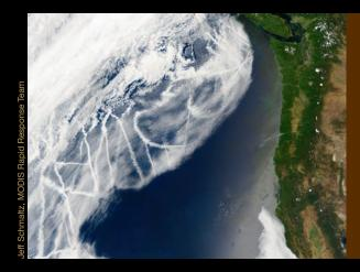
The satellite image shows an example of how clouds and aerosols interact. As ships cross the Pacific Ocean, their exhaust releases tiny aerosol particles around which water droplets aggregate, resulting in smaller, more numerous cloud droplets packed closely together. Thus, there are bright white streaks in the cloud where the ships' exhaust has intermingled with the surrounding stratiform cloud.
